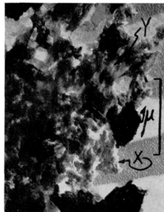
Fig. 1.—Electron micrograph, \times 20000 of SCHMIDT's aluminum hydroxide gel dried on Formvar from aqueous suspension and shadow cast with chromium at arctan 0.32 .
